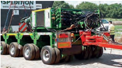
The PPU can be placed at the rear as well as on top of the vehicle
